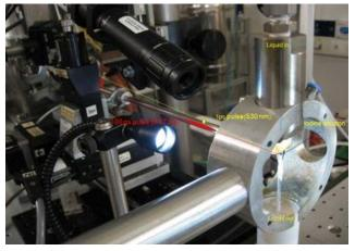
The experimental setup showing schematically the laser and x-ray pulse in space 100 picosecond before they strike the sample. The 100 ps x-ray pulse forms a 30 mm long needle with a 0.3 mm long laser pulse inside it. By varying the relative position of the pulses and using deconvolution algorithms, the distance between the iodine atoms can be measured with 10 ps resolution.
