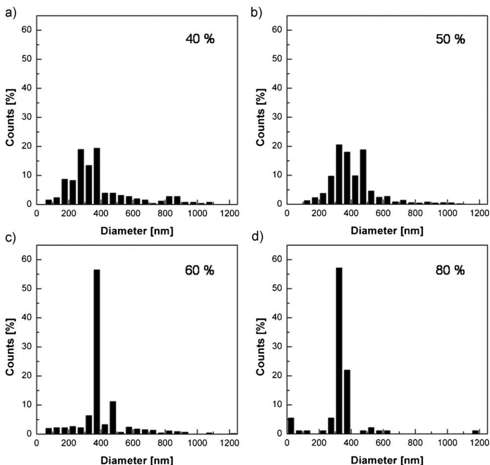
**Figure 5.** Histograms for the size distribution of bionanospheres at various humidity conditions: a) 40%, b) 50%, c) 60%, and d) 80%. The mean diameters of the spheres were approximately 379 nm, 399 nm, 397 nm, and 334 nm for (a)–(d), respectively.
