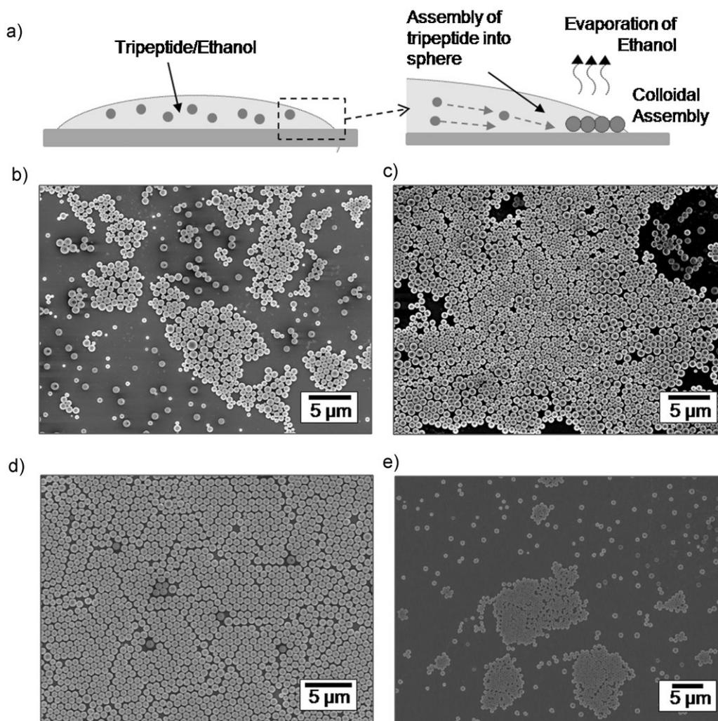
**Figure 4.** Hierarchical self-assembly of Boc-FFF into a hexagonal bionanosphere array at various humidity conditions. a) Schematic illustration of hierarchical assembly into a hexagonal bionanosphere array. During evaporation of the ethanol, Boc-FFF molecules assemble into bionanospheres that close pack to form a hexagonal array. SEM images of bionanospheres at relative humidities of b) 40%, c) 50%, d) 60%, and e) 80%.
