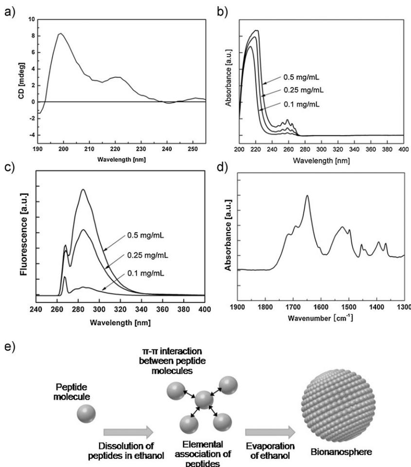
**Figure 2.** Spectroscopic analysis of the molecular interactions for a Boc-FFF assembly. a) CD spectrum, b) UV/Vis absorption, and c) fluorescence emission ( $\lambda_{\text{excitation}} = 260 \text{ nm}$ ) of dilute Boc-FFF solution. d) FT-IR spectrum of the dried bionanospheres. e) Proposed self-assembly mechanism. A phenyl ring of Boc-FFF undergoes  $\pi$ - $\pi$  stacking with a nearby phenyl ring from a neighboring molecule to facilitate assembly into a nanosphere morphology.
