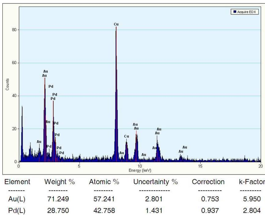
**Figure S5.** TEM-EDS analysis of a single AuPd alloy NW. Detailed analysis of several AuPd alloy NWs dispersed on the carbon coated copper TEM grid confirms approximately 1:1 atomic ratio of Au and Pd.
