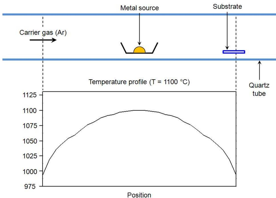
**Figure S6.** Experimental set-up used for synthesis of vertical Au, Pd, AuPd NWs. Shown below the furnace is the temperature profile, indicating that the centre of the heating zone is maintained at 1100 °C, whereas the substrates are at 1000 °C.
