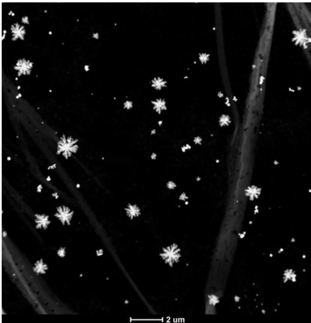
Figure S4. Six TEM images of the AuNPs in the sample solution collected in phase 1. Size histograms in Figure 2c were from these images. The particles have two different sizes ( \sim 950 nm and \sim 170 nm) and shapes (dendritic and spherical). Large rod-shaped structures of weak contrast in the background of the images are due to damages or impurities on the supporting carbon films of the TEM grid.
