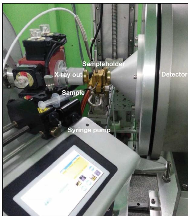
**Figure S1. Flow cell system for SAXS measurement at Pohang Light Source.** The sample is continuously injected using the syringe pump. The X-ray scattering pattern was measured using a quartz capillary in the flow cell available in the beamline.
